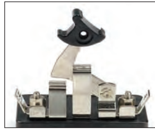
Safety-grip handle: A molded handle covers the terminal and includes a lower lip that projects over the metal parts of the switch, thus protecting the operator from contact with live components.
